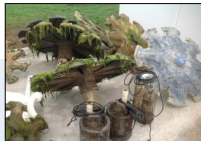
Algae and sediment residue on fountain intakes and underside of floats
